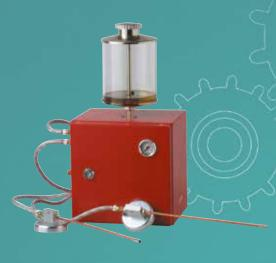
The liquid flows from the reservoir into a piston pump. This pushes an exact quantity of the lubricant into the internal feed tube. Separately supplied compressed air splits the medium at the nozzle tip and sprays it. External MQL in all metal-cutting operations. Pinpoint or small area lubrication in chipless forming operations. Application of mould release and anti-corrosion agents or other spray-on substances.
